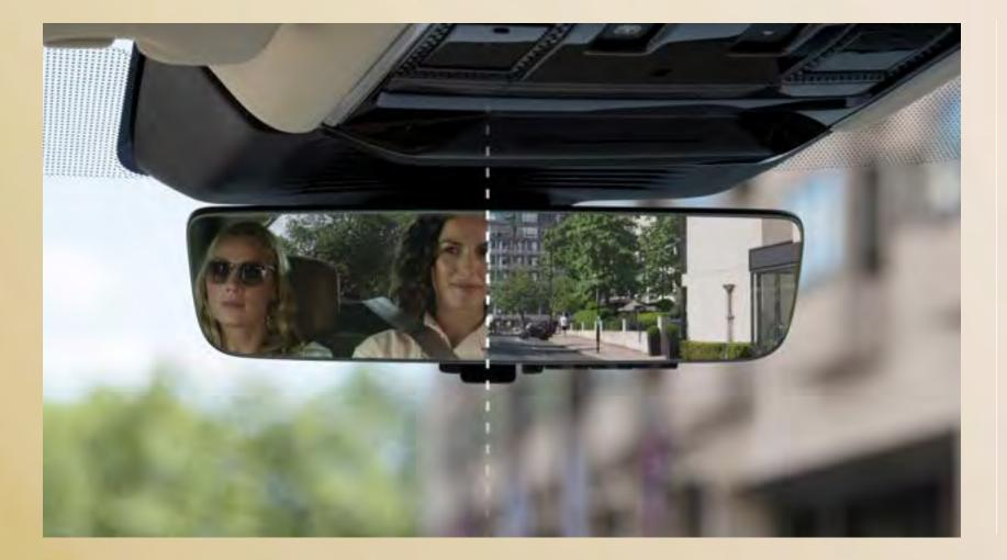
To maintain rearward visibility when carrying large loads or a full complement of seven occupants, Range Rover is available with ClearSight Interior Rear View technology<sup>9</sup>. At the touch of a button, the frameless interior mirror switches from a conventional mirror to a digital screen showing a feed provided by a high-definition rear-facing camera mounted
